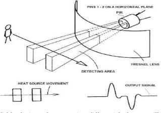
field of view, then negative differential change will be produced. PIR or Passive Infrared sensor is named as passive because it doesn't emit
